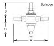
The temperature control valve between the vaporizer and service line regulator is designed to shut off the gas flow if the gas temperature drops below a pre-determined point, usually -20°F [144.4°K]. Such a temperature drop is often caused by a rapid or quick gas draw. If the temperature drops below the setting of the temperature control valve, the valve closes to prevent excessively cold gas from reaching the service end of the system. In particular, the cold gas is prevented
